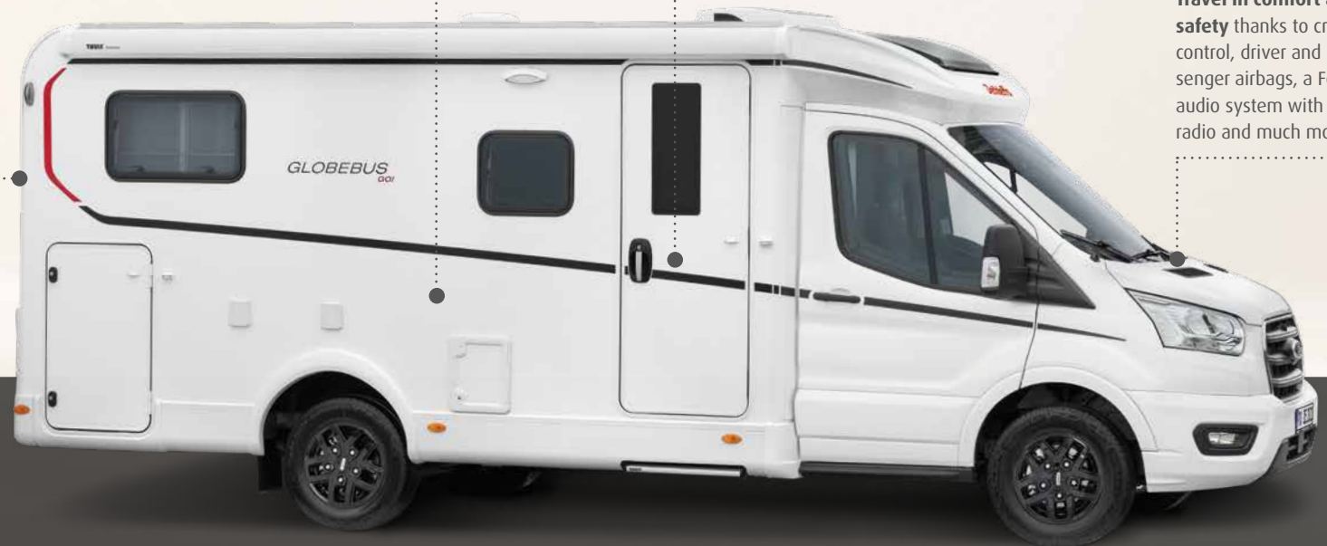
Roof, rear and side walls made of durable GRP
