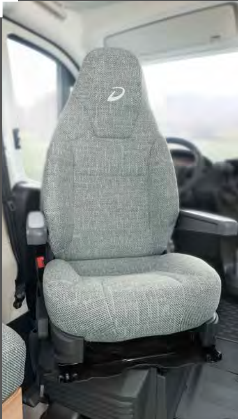
Ergonomic, swivelling CaptainChair seats with integrated headrest, two armrests and height/tilt adjustment
