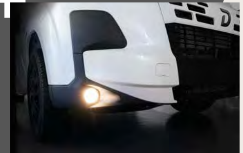
For a better view of the road: fog lights with cornering light feature
