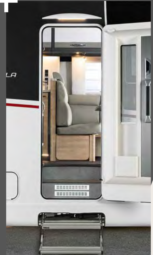
70 cm-wide habitation door with window, central locking system and electric closing aid
