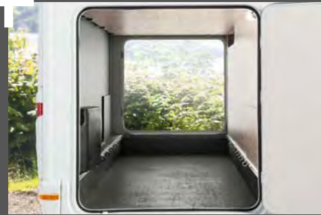
Large rear garages with access from both sides and smooth-running twist/quick-release latches.
