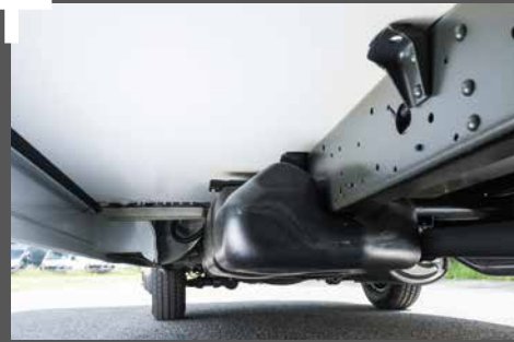
Durable, Lifetime-Plus bodywork construction without wood inserts! GRP-clad underfloor
