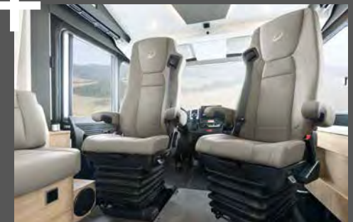
Travel first class thanks to shock-absorbing hydraulic seats with a heated and ventilated seat surface (option)
