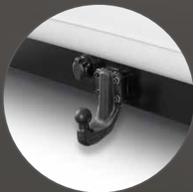
Towing capacity 3.5 t braked; tow bar (optional)
